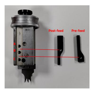
Moving the post-feed cam from B to A changes the stroke from 40 to 30 mm. Moving the pre-feed cam from C to B changes the stroke from 40 to 30 mm.
