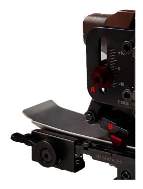
For adapting the pawl B to the pitch of the terminals, in order to have a new terminal correctly placed on the anvil for each cycle of the press: loosen the nut A and move the screw up for a greater pitch or down for a shorter one. Then tighten the nut again.
