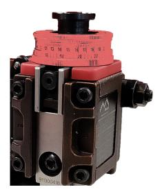
Free the brake by means of the lever B, place the terminals in the guide A, push it until it will be hooked by the pawl C and then tighten the brake by means of the lever B.
