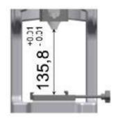
Verify that the press and the mini applicator's axis are perfectly in line.
