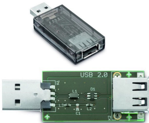
Figure 24: USB Dongle, closed and opened, layout according to Figure 23, circuit diagram according to Figure 13.
