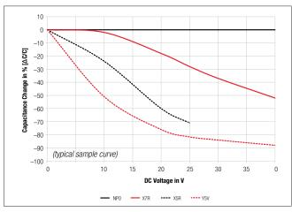
\*Typical characteristics for ceramic capacitors with a rated DC voltage of 25 V (X5R) and 50 V (NP0, X7R, Y5V)
