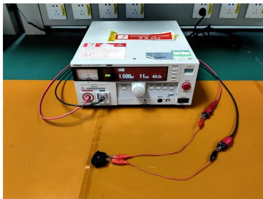
耐电压 Withstand voltage (pin-pin)
