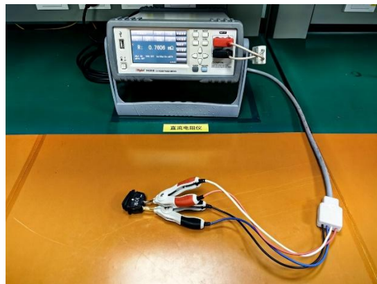
接触电阻 Contact Resistance
