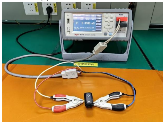
接触电阻 Contact Resistance
