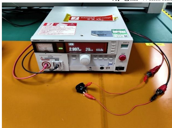
耐电压 Withstand voltage (pin-case)
