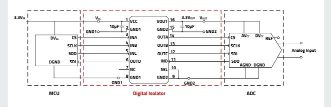
• SPI interface for communication between the analog-to-digital converter and MCU
