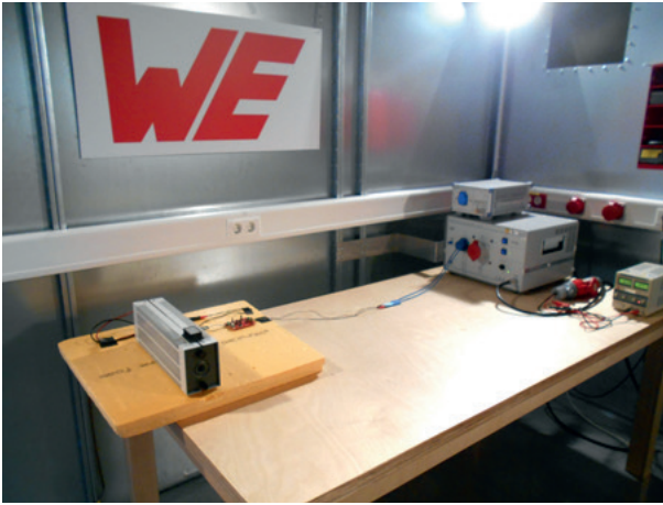
Fig. 15: CISPR-32 Conducted emissions setup
