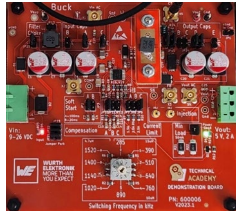
Figure 10: Buck Converter for the test.
