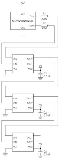
The information of each LED is transmitted with Most Significant Bit (MSB) first.
