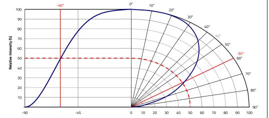
Viewing Angle - Phototransistor
