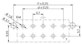
Recommended PCB Layout Thickness: 1.6mm General Tolerance ± 0.05 mm
