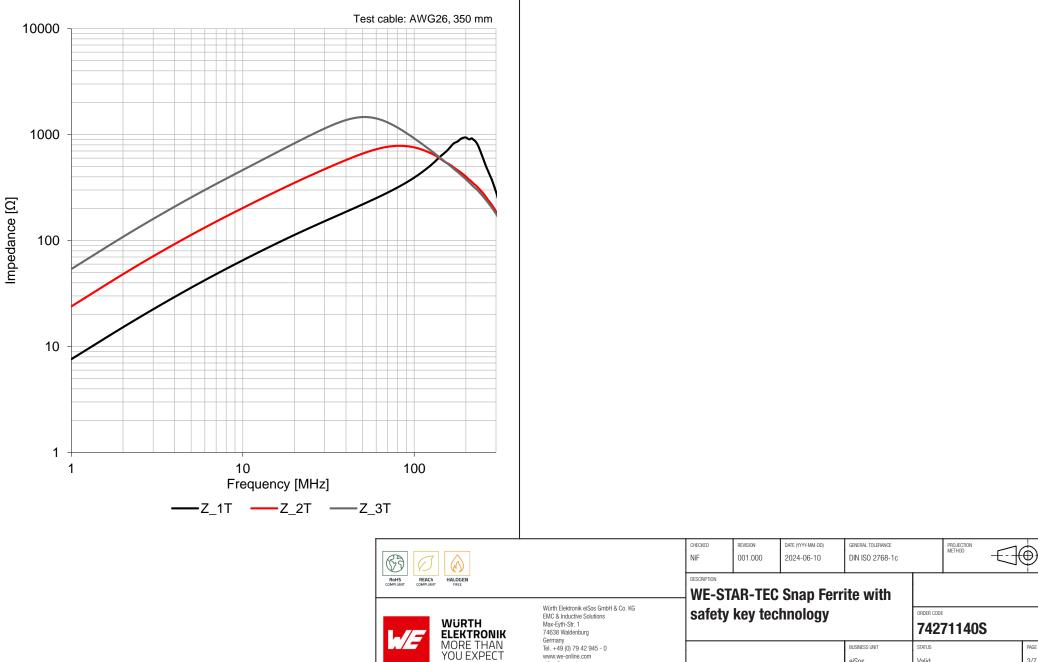
**Typical Impedance vs. Frequency Characteristics:**
