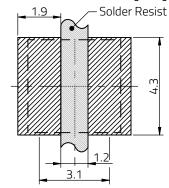
Landing pattern based on IPC-7351 Standard No vias and traces underneath the inductor 6:1
