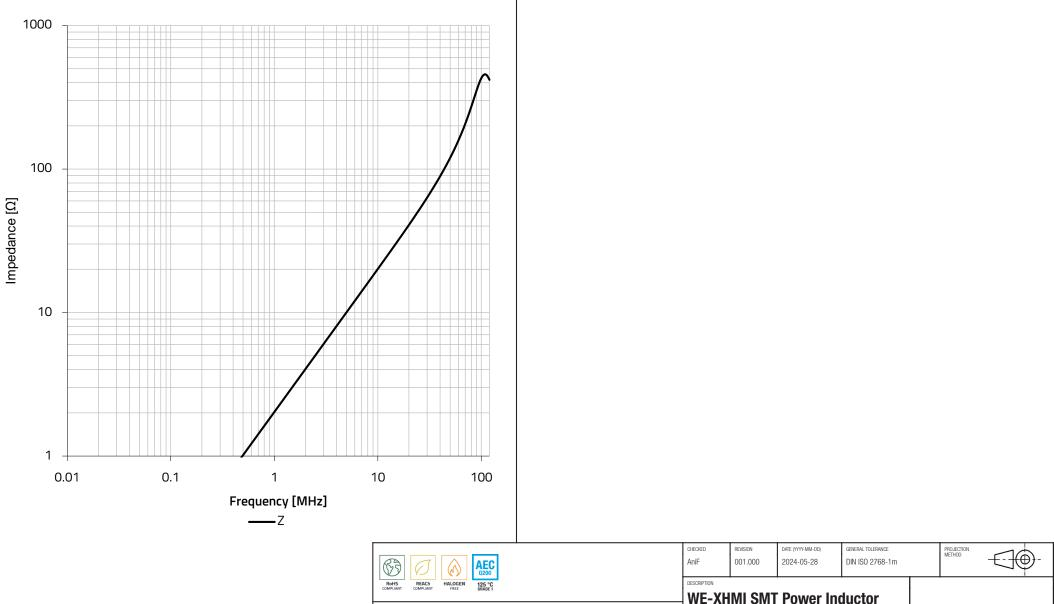
**Typical Impedance vs. Frequency Characteristics:**
