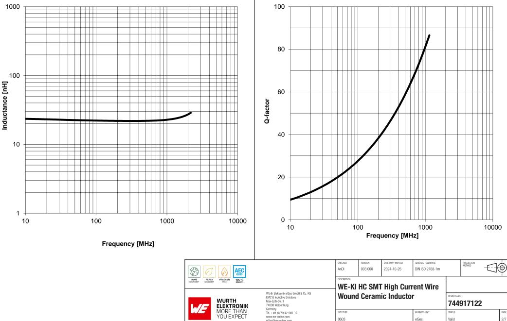
**Typical Inductance vs. Frequency Characteristics:**
