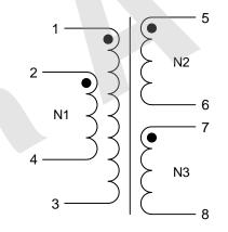
Application of the transformer allows for the leadwires between terminals 1&2 and 3&4 to solder bridge.
