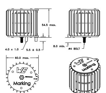
Bolt used only for mechanical stability
