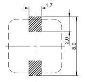
no sensitive traces underneath the component
