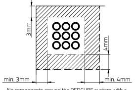
No components around the REDCUBE system with a minimum safety distance of 4mm
