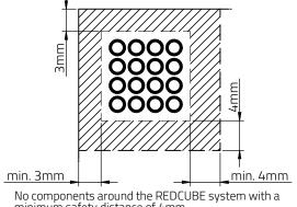
No components around the REDCUBE system with a minimum safety distance of 4mm
