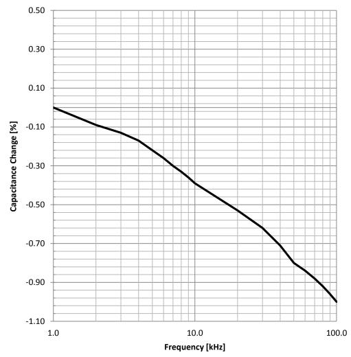
Test Equipment: E4991A or equivalent
