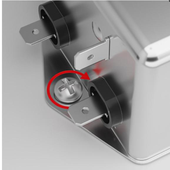
To establish a low impedance path for parasitic currents, the filter housing shall have a wide connection area to the ground plane. The ground plane shall be free of paint or other isolating materials.
