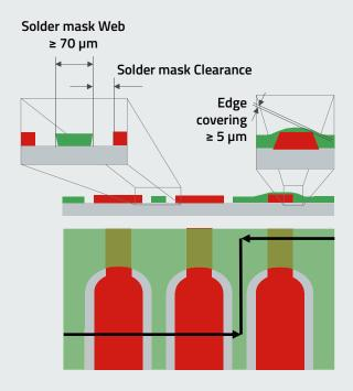
Our standard for soldermask is green photosensitive soldermask that meets the requirements of IPC-SM-840 Class T and H. Other colors such as white, black, blue, red or yellow can also be applied on request. Depending on the production location, the execution is as a colored solder mask instead of the green solder mask or as an additional print over the standard green solder mask. Please ask for these options, we will provide you with a quote.
