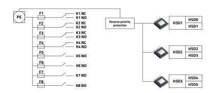
Design has an internal parallel diode on each coil. We recommend using relays with diode or no protection at all. Relays with resistor are generating more heat within the enclosed environment.
