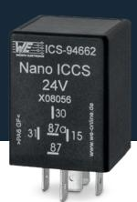
The **Nano ICCS** are small and powerfull controllers shaped as relays with 5 or 6 pins. They can be connected to the circuit board using standard relay sockets.
