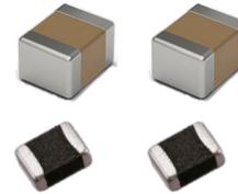
The varistor protects the capacitors from damage caused by transient overvoltages.
