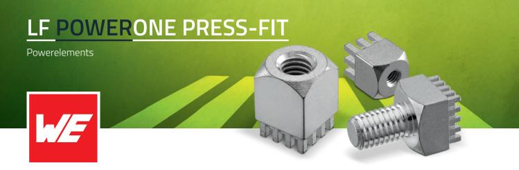
**LF PowerOne Press-Fit** Powerelements are one-piece lead-free high current contacts in solid design which are used for the supply and distribution of high currents to PCBs. They are flexible, configurable, and easily usable in thousands of various designs. Depending on the pin arrangement and the layout, currents of up to 1000 amperes are possible. This makes these power supply terminals ideal for use as connection elements for fuses, for cable connections to the PCB, or as fastening elements.
