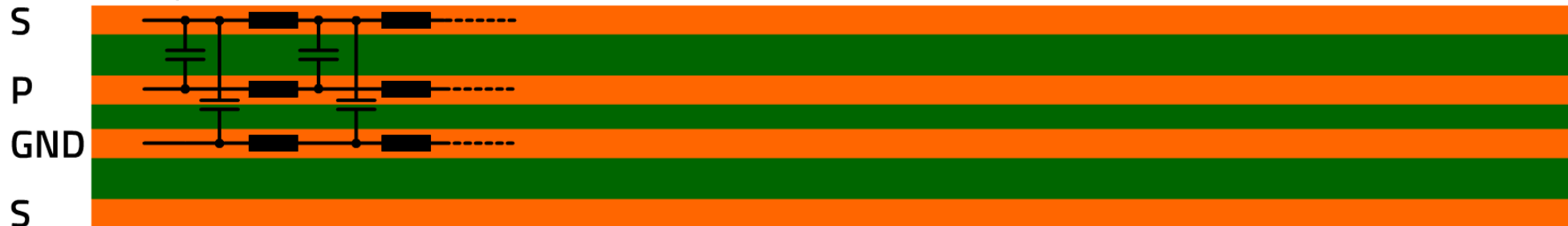
4 layer PCB transmission line
