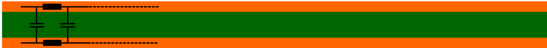
2 layer PCB transmission line
