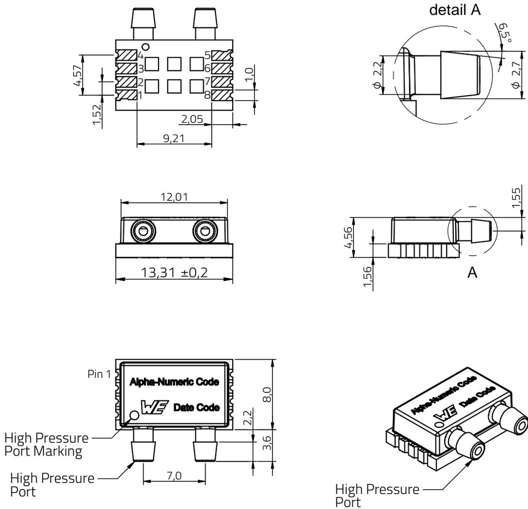
Figure 12: Sensor dimensions: Horizontal-barbed nozzles [mm]
