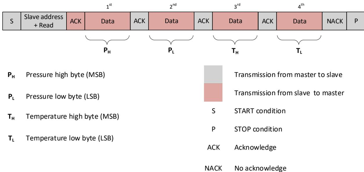
Figure 10: Reading output data with I<sup>2</sup>C interface
