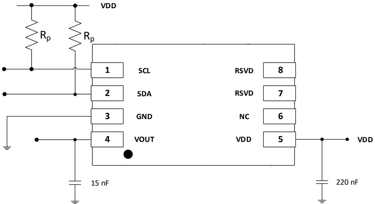
Figure 9: Application circuit with I<sup>2</sup>C interface (top view)
