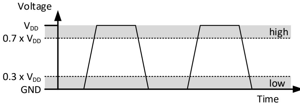
Figure 5: *SDA* and *SCL* logic levels
