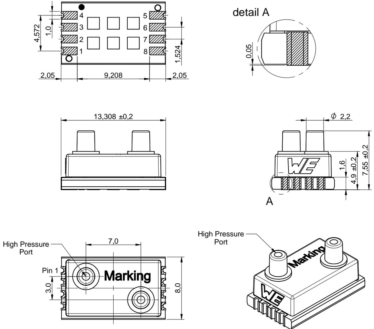
Figure 11: Sensor dimensions: Vertical nozzles [mm]
