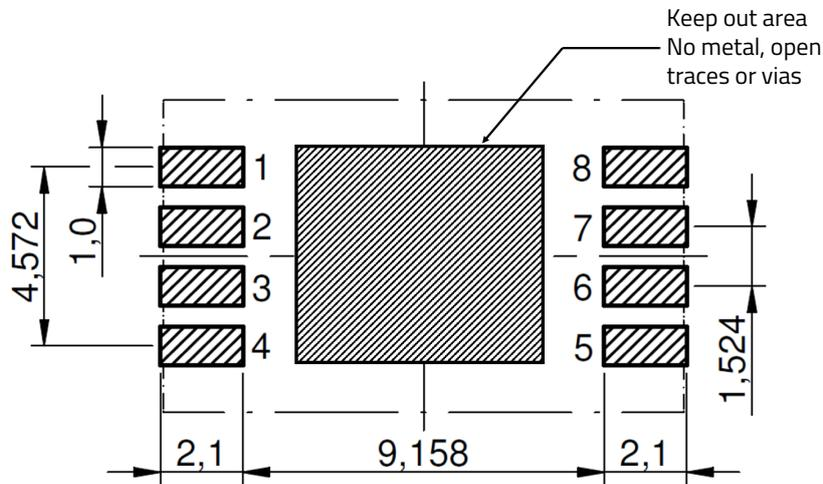
Figure 13: Vertical nozzles: Recommended land pattern [mm] (top view)
